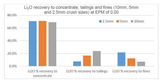
Figure 14: Li<sub>2</sub>O recovery to concentrate, tailings and fines at the three crush sizes.
