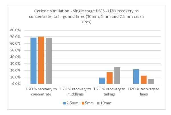
Figure 16: Cyclone simulation results showing Li<sub>2</sub>O recovery to concentrate, tailings and fines at the three crush-sizes for single stage DMS.
