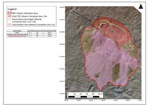
*Figure 20: Survey plan and model used in calculating the resource volume.*
