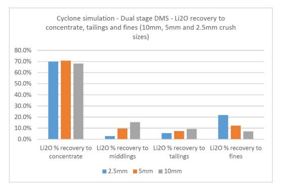
Figure 15: Cyclone simulation results showing Li<sub>2</sub>O recovery to concentrate, tailings and fines at the three crush-sizes for dual stage DMS.
