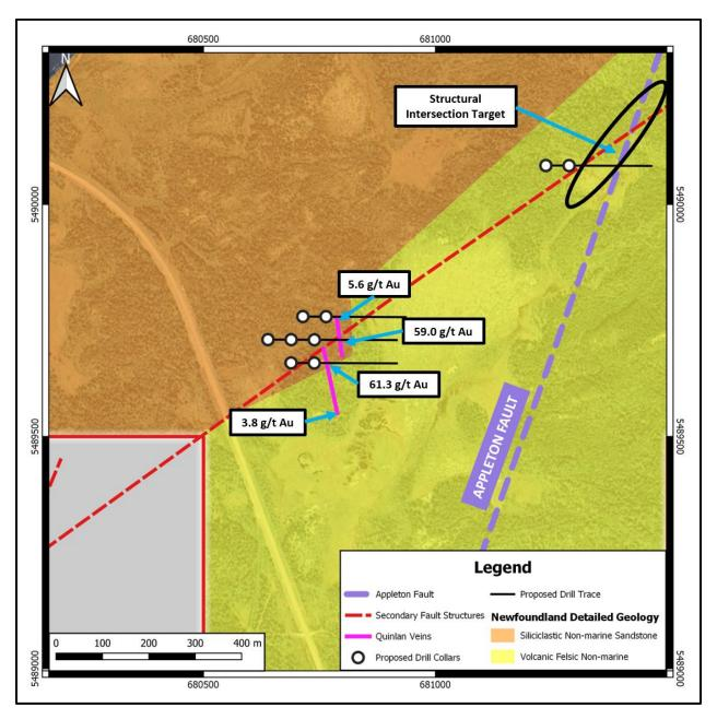
**Figure 2:** Geologic map of the Quinlan Veins prospect with proposed drill collars and identified gold in quartz veins (pink lines) and locations where samples up to 61.3 g/t Au were collected. The veins are believed to be associated with the Appleton Fault zone and its secondary fault splays, with the intersection identified by Goldspot being a high priority target as well.
