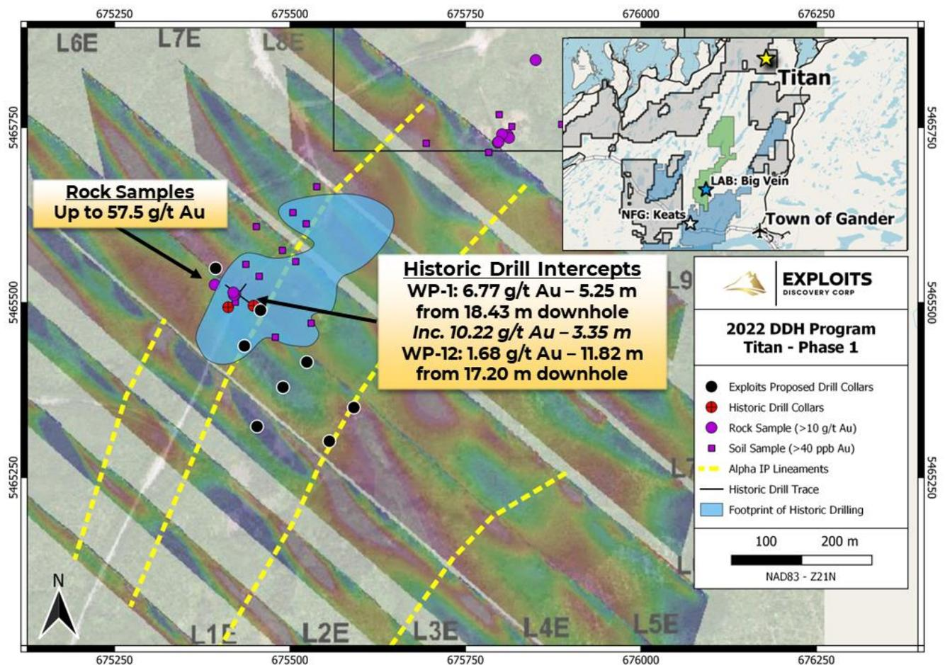
**Figure 1:** Historic drilling and 2022 Phase 1 proposed drill collars overlaying 3D image highlighting Alpha IP lineaments from vertical profiles.
