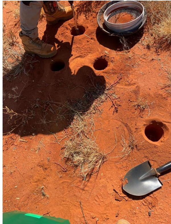
Note: Auger holes and sampling on the auger traverse at Isbjorn Project
