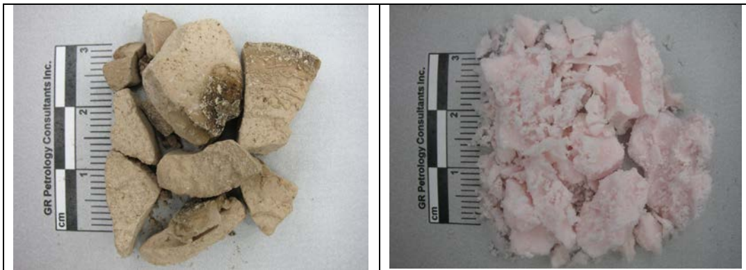
Fig. 2: Lithium carbonate and lithium chloride solids recovered from processing Sturgeon Lake brine.
