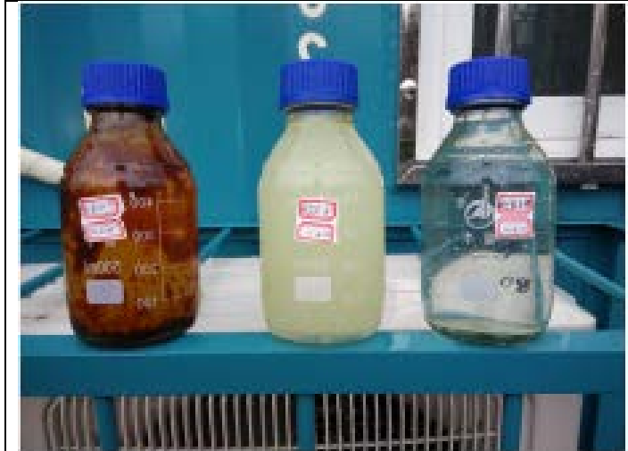
Fig. 3: Jinan Refinery Pilot Test – Raw water into Induced Gas Flotation unit, Treated water with emulsified oil after IGF and treated water after RSL membranes™.
