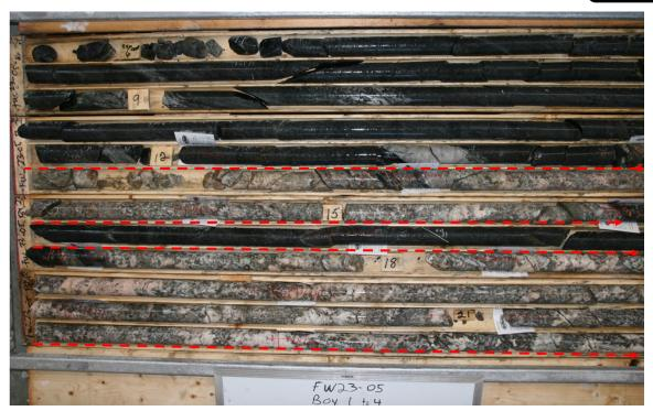
Figure 1. Borehole FW23-05 Core Samples showing high-grade (>1.3% Li₂O) spodumene mineralization (Far West South "FWS" Pegmatite)
