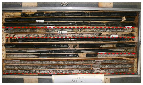
Figure 2. Core showing high-grade (1.5% Li<sub>2</sub>O) spodumene mineralization in Hole FW23-07 (Far West North "FWN" Pegmatite)
