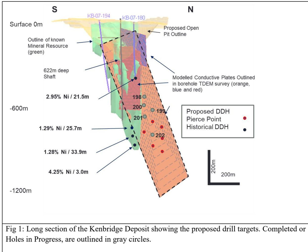
Fig 1: Long section of the Kenbridge Deposit showing the proposed drill targets. Completed or Holes in Progress, are outlined in gray circles.
