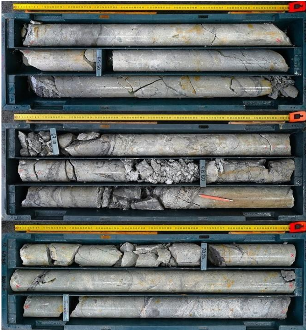
Figure 1. Photograph of PQ3 diameter core between 64.3 and 72.4m downhole in CMV25001. Dark sulphide veining and breccia cement can be observed, correlating to the reported mineralised interval ( click here to view image ).
