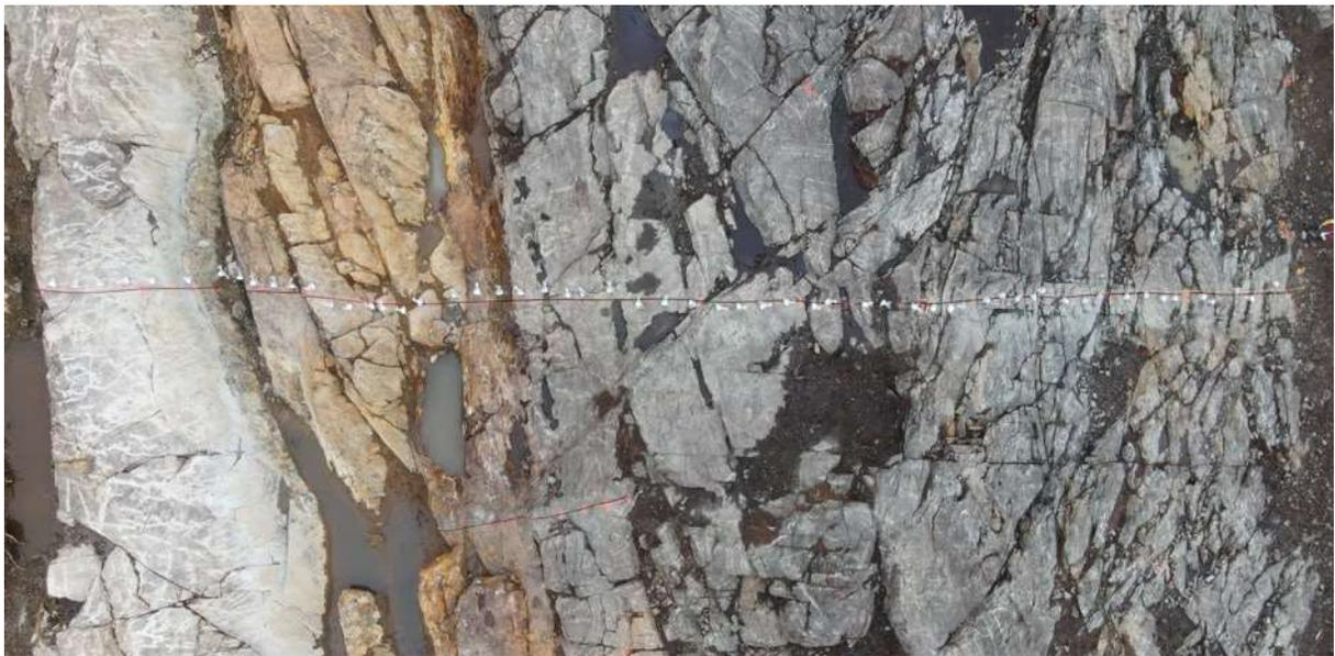
39.4m channel viewed from above, cut, bagged, tagged and sealed in the field. The southern ultramafic band is in the left, the oxidized main deformation band is rust coloured in the centre and the northern ultramafic band, which is the better mineralized of the ultramafic bands, is on the right.
