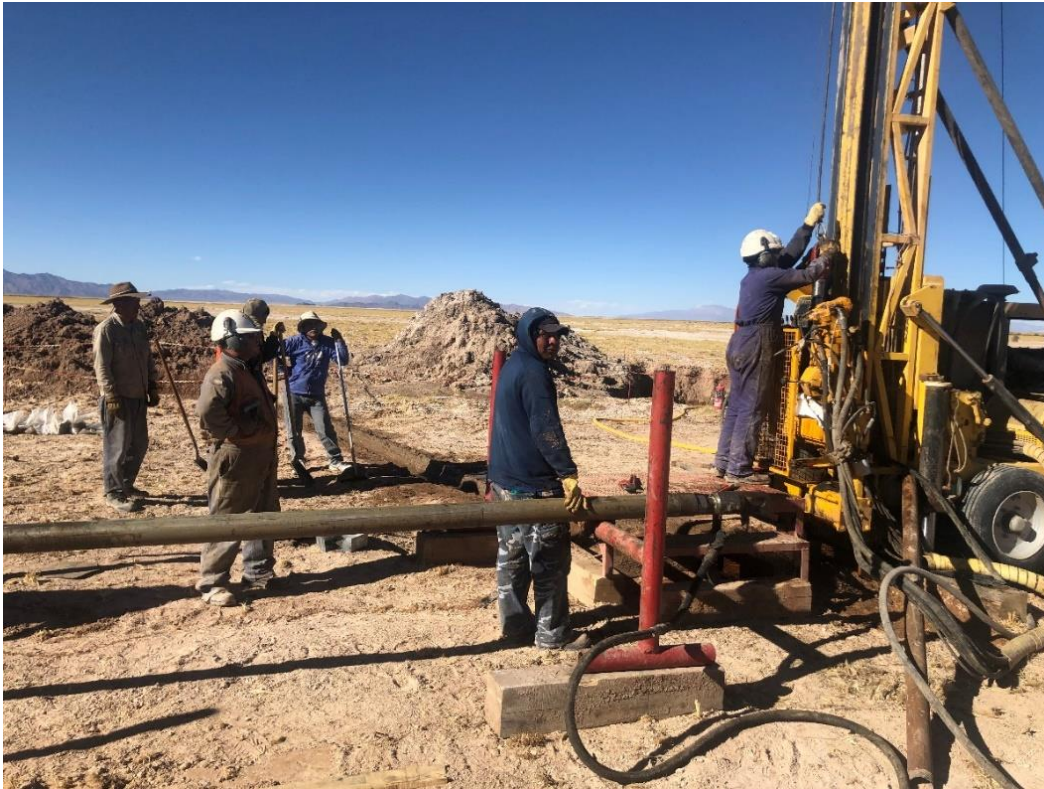
Figure 1. Drilling of 6-inch well for steel casing prior to HQ diamond drilling. Casing prevents collapse of well in unconsolidated sediments as brine pressures at depth are significant.
