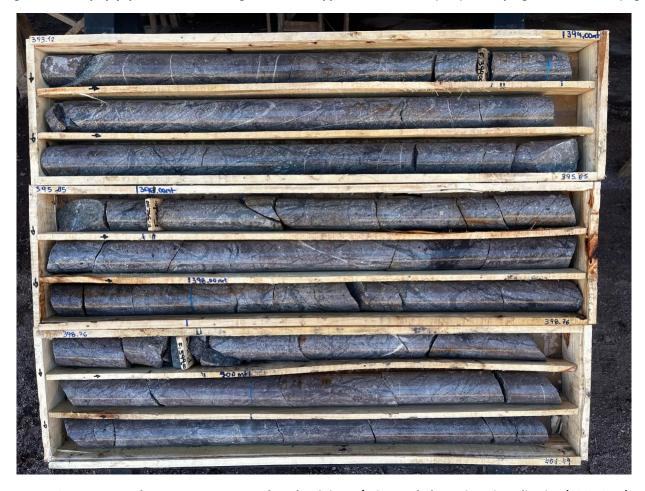
Image 3. Intense Porphyry A type quartz stockwork veining w/primary chalcopyrite mineralization (393-401m)
