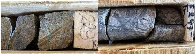
Images 1 & 2: Porphyry qtz stockwork veining with oxide copper mineralization (Left) and supergene enrichment (Right)
