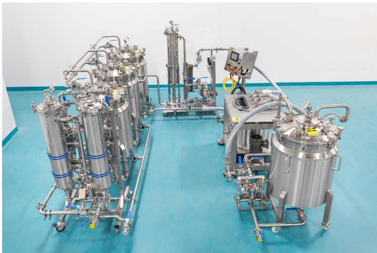
Figure 1 - Cryo-Ethanol Extraction System
