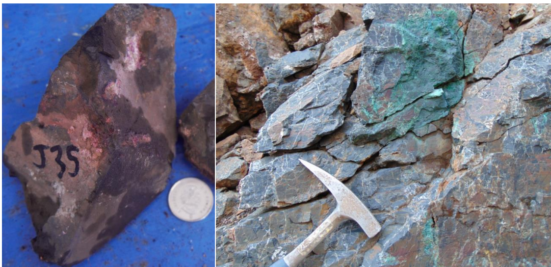
Figure 1. Left, Sample J35, a dolostone with erythrite staining. This sample yielded 2.96% Co. Right, Malachite staining in the Mark’s Hi-Grade showing.
