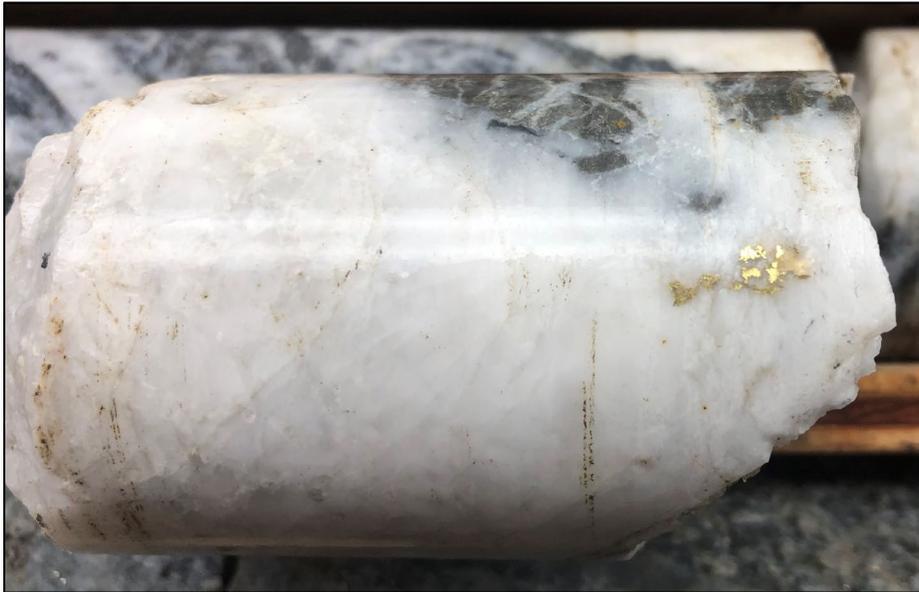
**FIGURE 3 – Visible Gold in Drill Intercept I-19-13 (in retained half core)**
