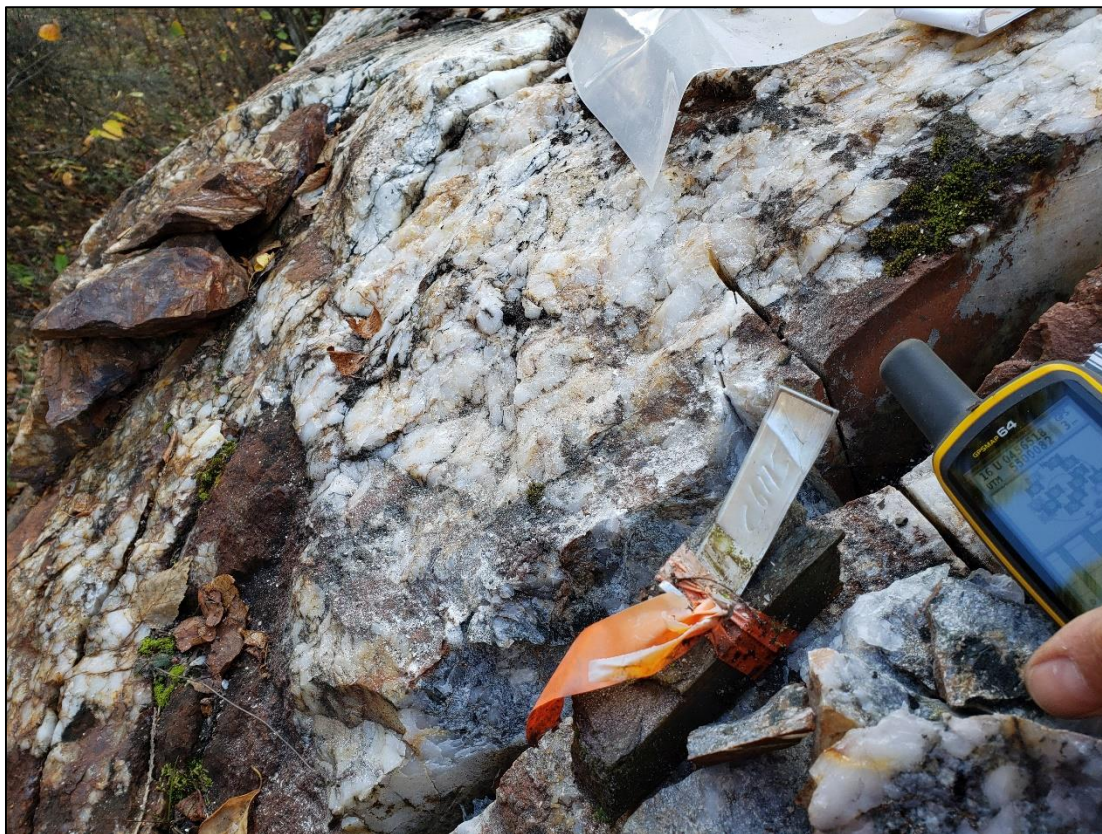
Figure 11. Glassy grey to white quartz veining with arsenopyrite mineralization noted in the Dumont trenching efforts by Prodigy Gold, 2010 (the Issuer, 2020).
