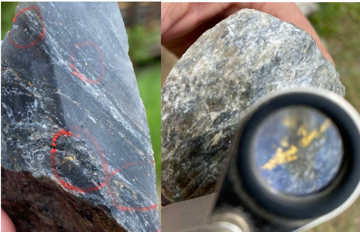
Figures 1 & 2 - Close-ups of the VG identified in intervals from two holes
