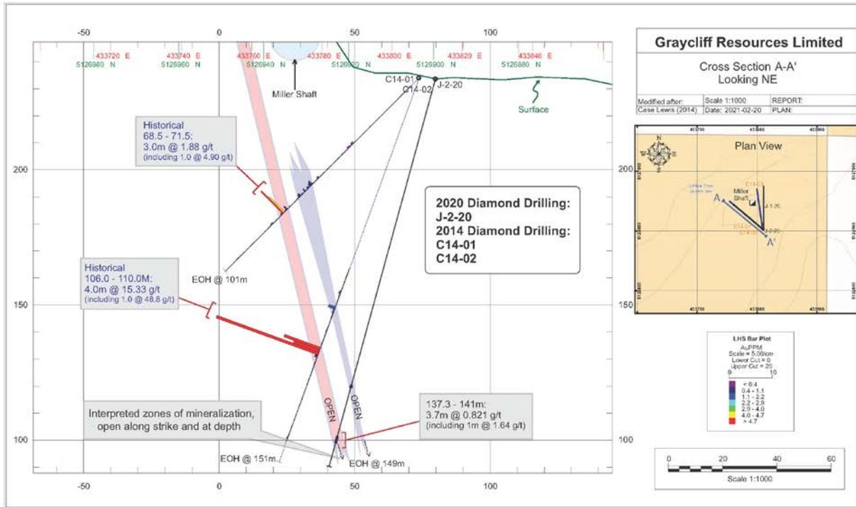
Figure 2 - Cross Section A-A'
