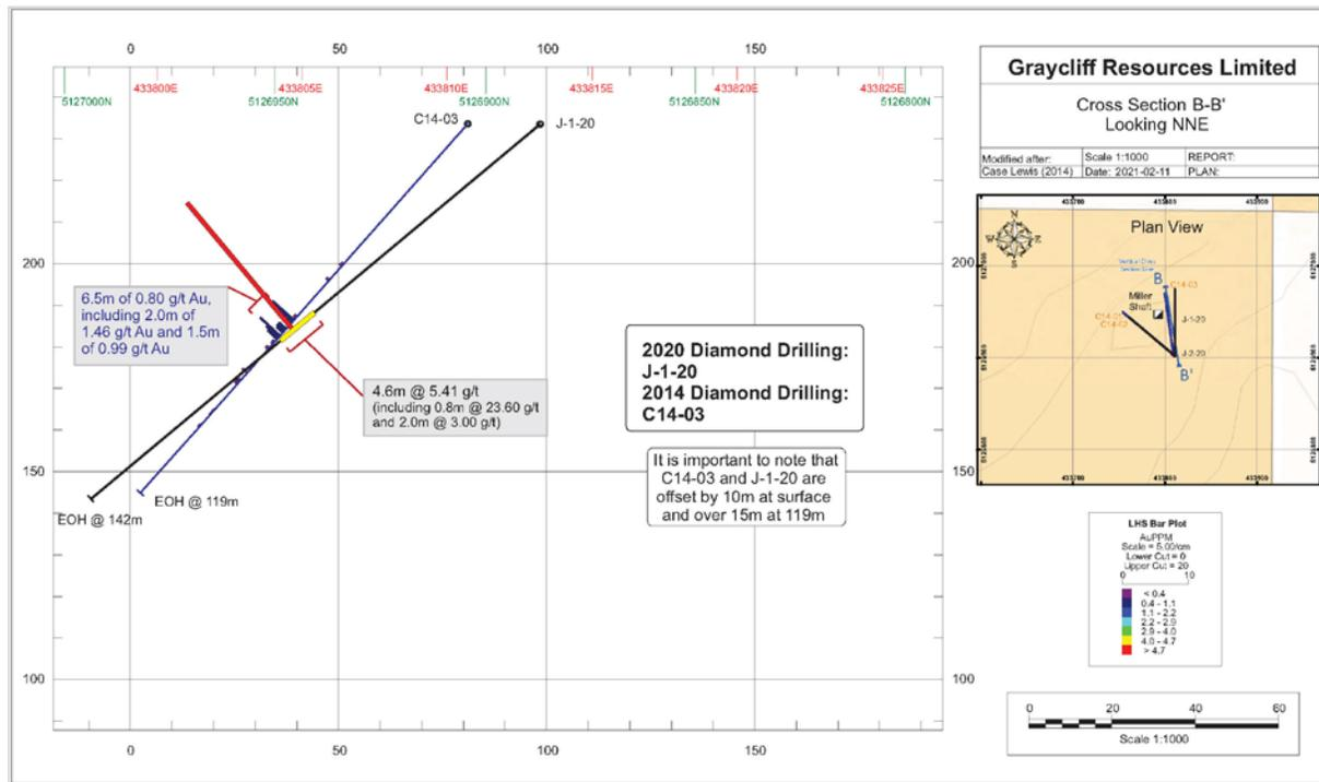
Figure 3 - Cross Section B-B'
