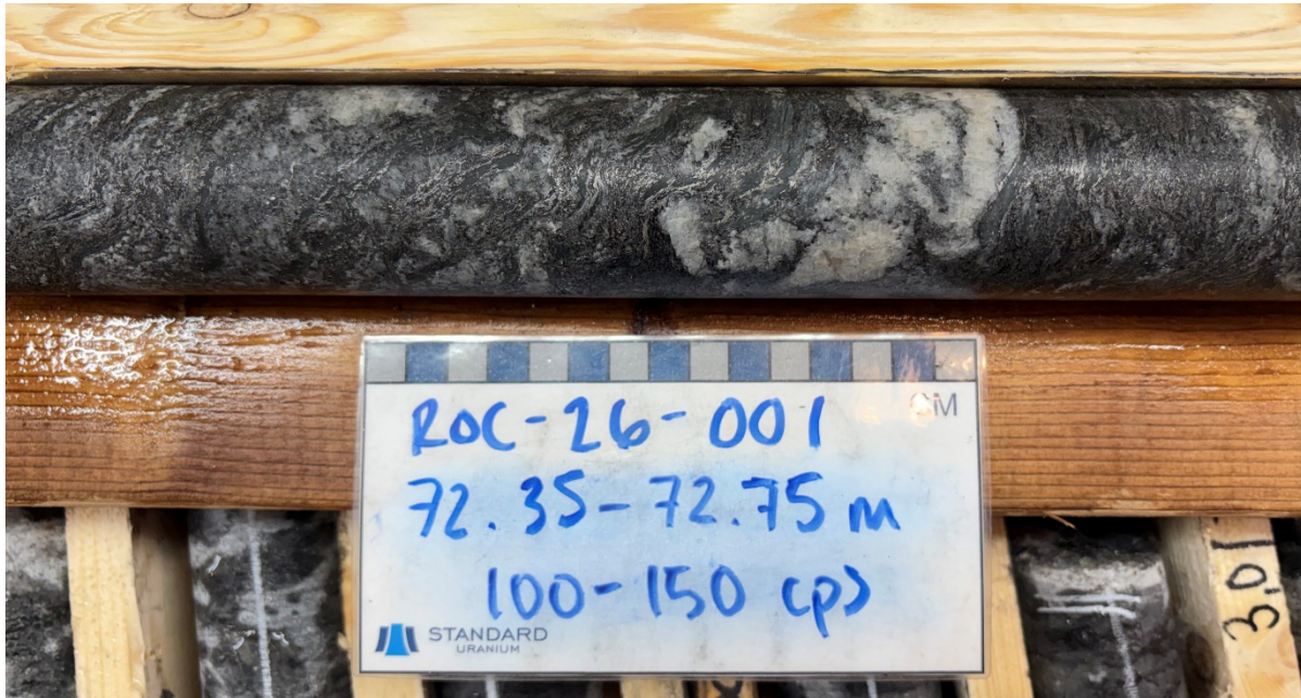
Figure 3. Drill core photo of chloritized graphitic pelitic gneiss in ROC-26-001
