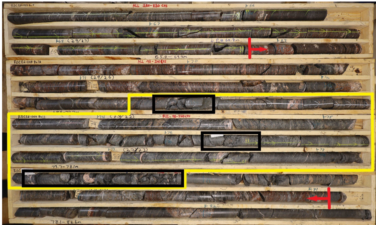
Figure 3. Drill core photo of chloritized graphitic pelitic gneiss in ROC-26-001
