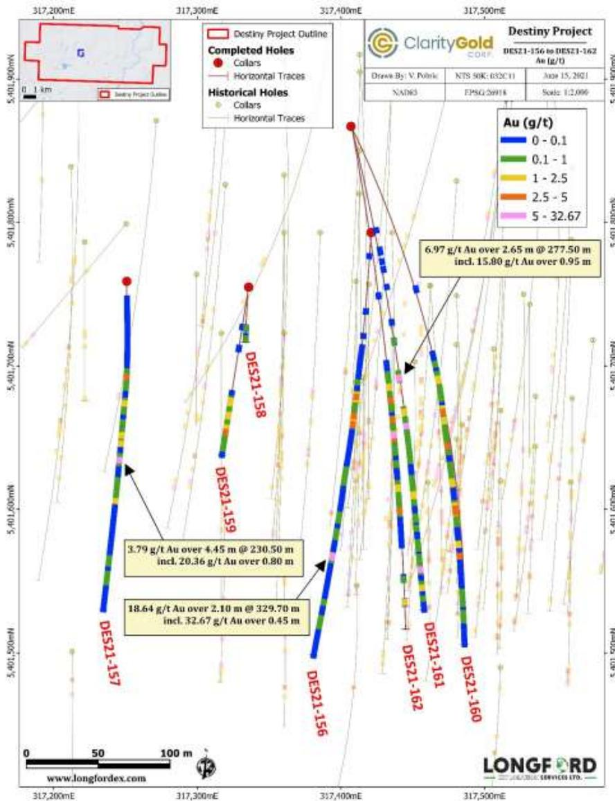
Figure 2 - Plan map showing Results from DES21-156 through DES21-162 including historic drill intercepts.
