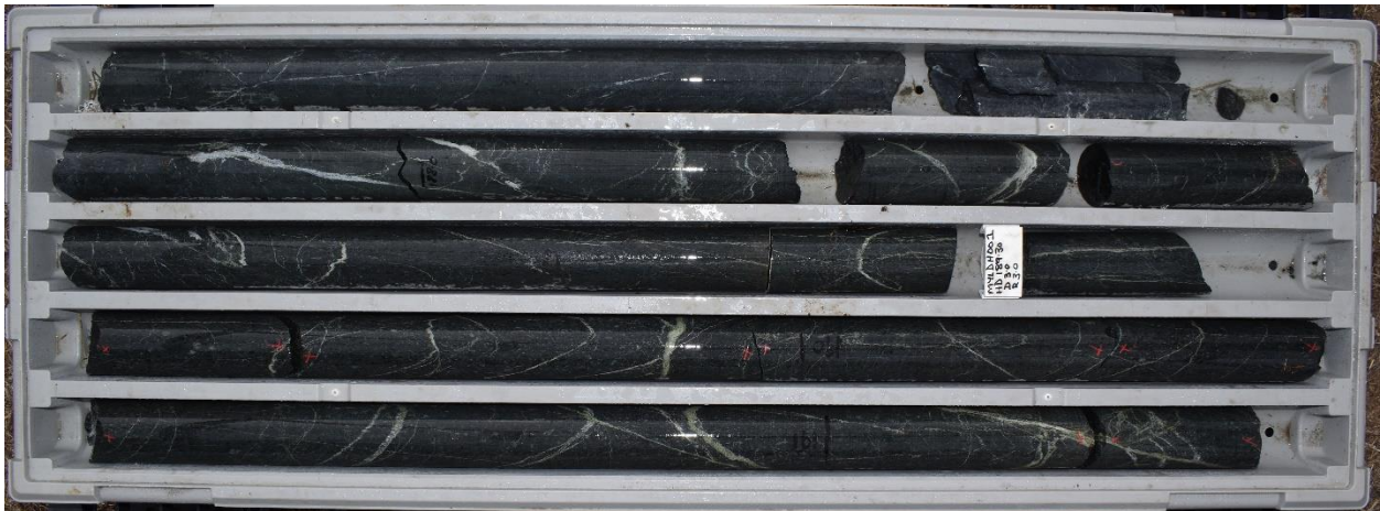
Photo 1: Myallmundi drill hole MYLDH001– 186.87 to 191.34 meters. Strongly biotite-magnetite altered basalt crosscut by several generations of vein stockwork comprising chlorite-magnetite, quartz-carbonate and epidote-quartz carbonate.
