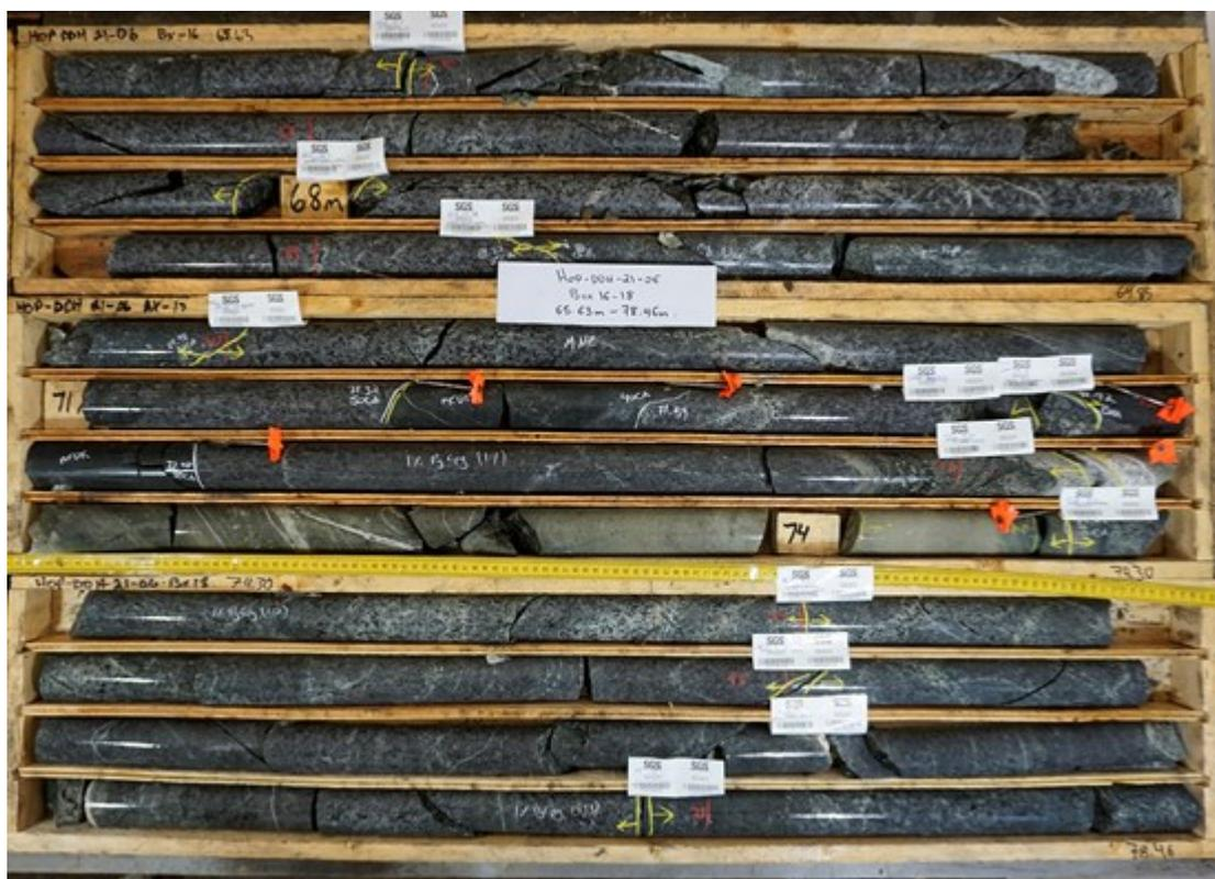
Figure 2. Drill core from HOP21-DDH-06 displaying mineralized intersection from 65.63m - 78.46m which partly falls within 13.69m (69.98m - 83.67m) of 0.400% Cu.
