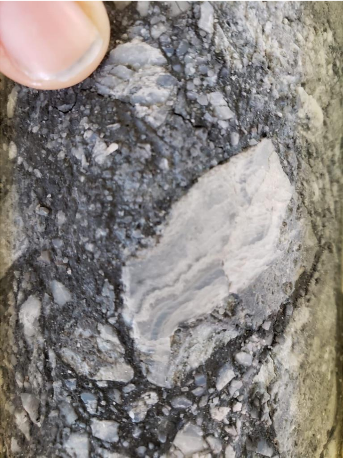
(Figure 2: Example of vein breccia from hole 19OMS-003. Vein fragments are finely banded, typical of epithermal veins. Dark matrix material is rich in pyrite.)
