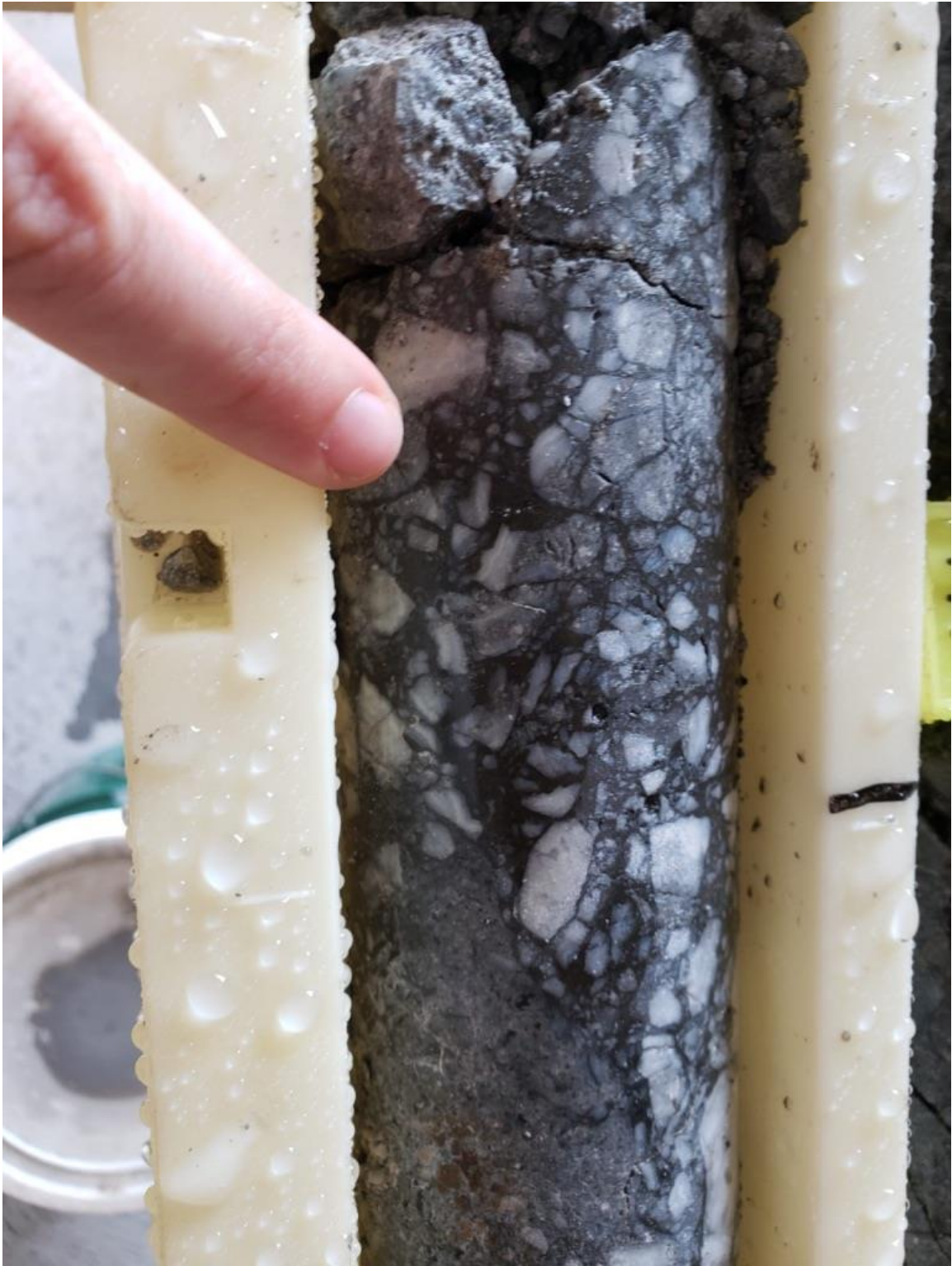
(Figure 3: Example of intensely silicified vein breccia from hole 19OMS-003. Quartz vein fragments are floating in dark gray, pyrite-rich silica.)
