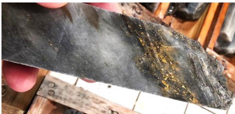
Picture 1 - Drill Core from sample at 123 m - 124 m showing Visible Gold
