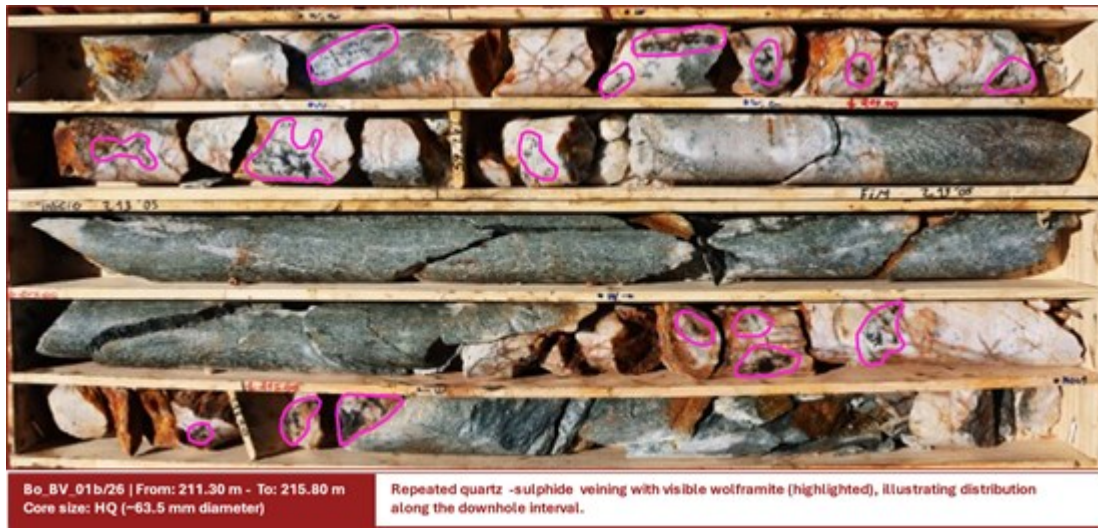
Figure 3 (above): Drill core from hole Bo_BV_01b/26 showing repeated occurrences of quartz-sulphide veining with visible wolframite tungsten mineralization (highlighted), demonstrating the distribution and continuity of mineralization along the downhole interval.
