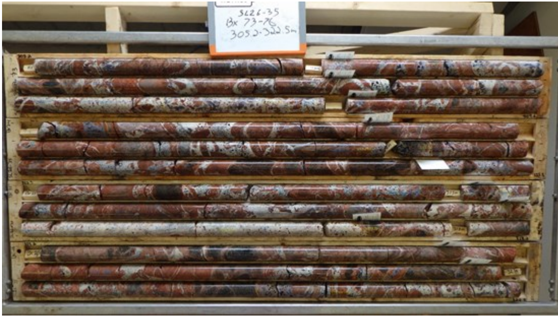
Figure 3. Abundant carbonatite mineralization veins (white rock) within syenite (orange rock), SL26-35, boxes 73-76 (305.2m-322.5m).
