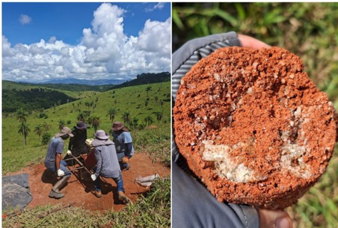
Figure 2: Auger drilling at Penelope (left) and REE-enriched regolith core (right).
