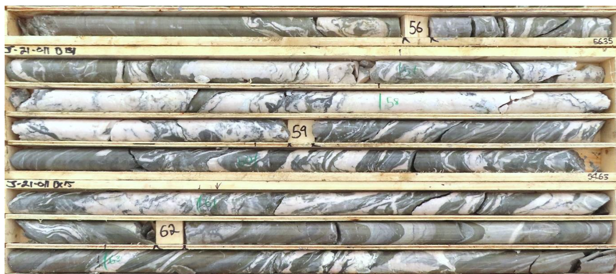
Figure 2 – Quartz flooding in a possible parasitic fold nose in J-21-011. Assays for the 5.0 m interval from 56.0 m to 61.0 m depth averaged 10.43 g/t Au (maximum 13.05 g/t Au), within a broader zone of 5.35 g/t Au over 12.5 m. Given the low angle of some beds to core axis, rough estimates of true thickness vary between 50-70% of reported intervals, though the geometry is not yet well constrained.
