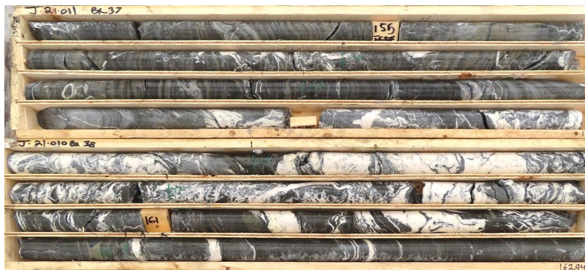
Figure 3 – Quartz flooding and brecciation in J-21-011. Assays for the 6.5 m interval from 155.5 m to 162.0 m depth averaged 13.2 g/t Au within a broader zone of 15.0 m averaging 5.97 g/t Au. These values are affected by a high-grade zone over 1.3 m from 159.5 m to 160.8 m which averaged 43.5 g/t Au. A 2-3 cm zone of massive arsenopyrite occurs within a 0.3 m assay interval from 160.5 m to 160.8 m which returned 63.9 g/t Au. Given angles observed in core, rough estimates of true thickness are 70-90% of reported intervals, though the geometry is not yet well constrained.
