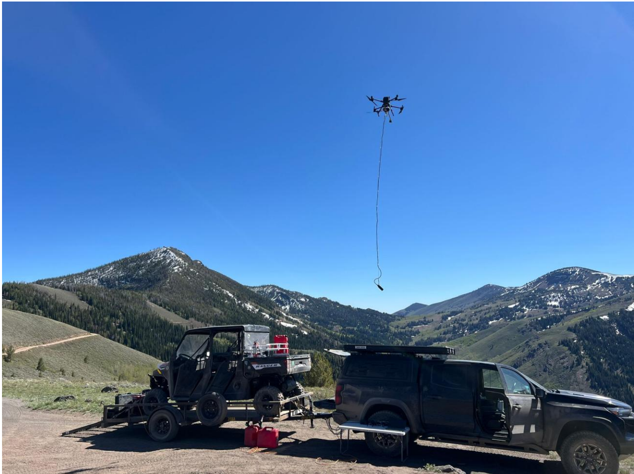
Figure 1: Field photograph of drone and magnetometer equipment being deployed at the Rowland Tungsten Property.
