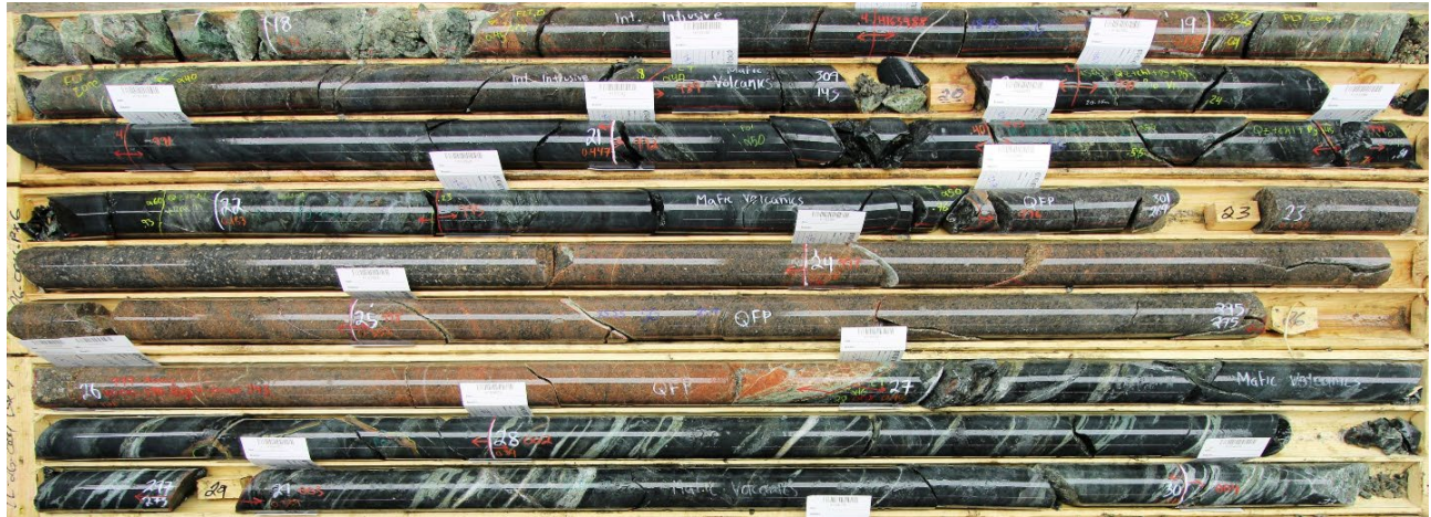
Figure 4: Altered and mineralized mafic volcanics from LL-26-004. Altered quartz-feldspar porphyry and fault zone also pictured.
