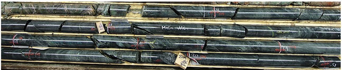
Figure 3: Sheared, silica-diopside flooded mafic volcanic with visible gold at ~18.75m in drill hole LL-26-005.
