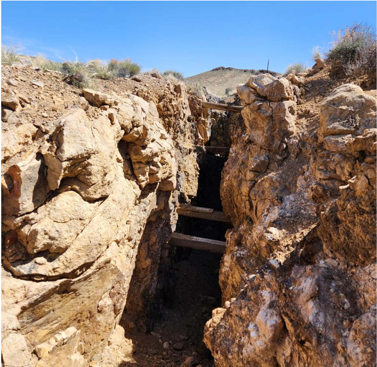
Figure 4: Historic workings likely targeting structurally controlled mercury mineralization associated with silicification and clay alteration. Open stope is approximately 1 metre in width.
