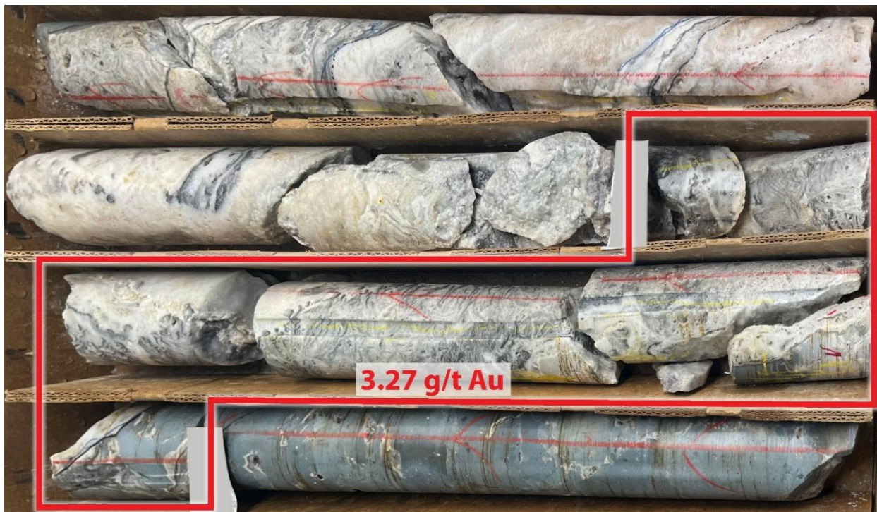
Figure 3: Photograph of 3.27 g/t Au over 0.88 m vein intercept in TJ25-01 showing abundant lattice-bladed quartz-after-calcite, vein sediments, and crustiform banding along the wall rock margins.
