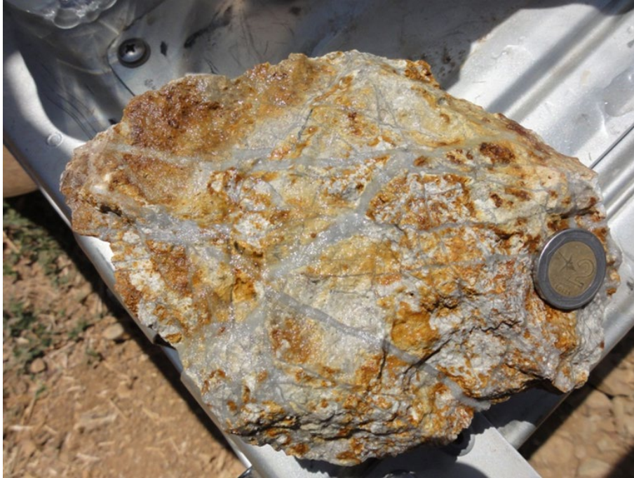
Figure 3: Dense A-vein stockwork within a potassic altered dacitic tuff At the Cerro Quillo Porphyry Au-Cu-Mo Prospect.
