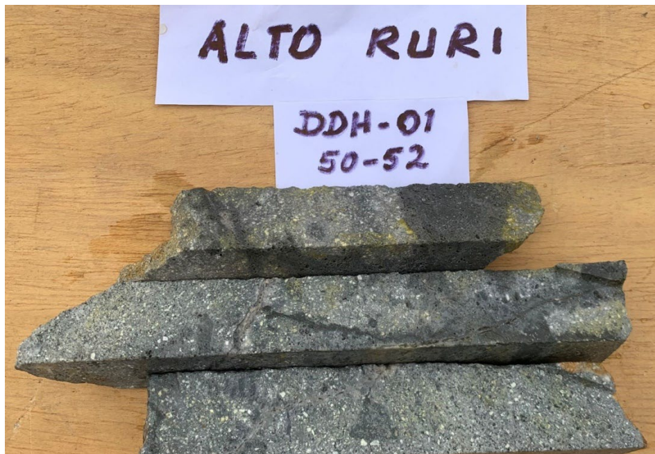
Figure 2: Drill core from Alto Ruri hole AR001 showing irregular vuggy silica replacement of advanced argillic altered volcanoclastic rock.
