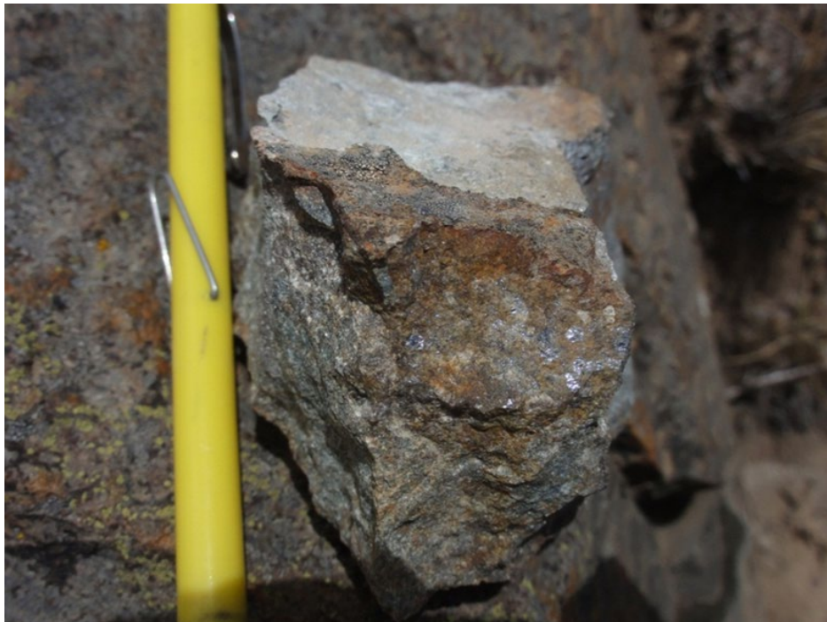
Figure 4: A type B-vein with disseminated molybdenite crosscutting a dacite pyroclastic tuff at the Cerro Quillo Porphyry Au-Cu-Mo Prospect.
