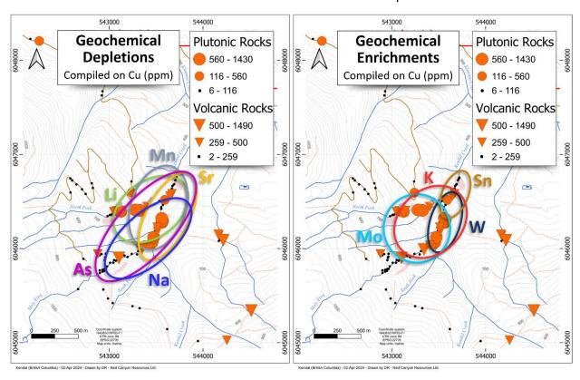
Figure 5: Maps showing compiled geochemical distributions of depleted (left) and enriched (right) elements summarized by ellipses on top of the map showing copper enrichments. The 800 x 500 metre region of Cu enrichment is overlain by coincident depletions in Na, As, Sr, Li and Mn and enrichments of K, Mo, W and Sn. Importantly, there is a >700 m sampling gap to the east of the ellipses.
