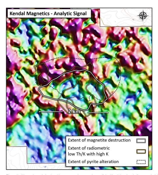
Figure 7: Magnetic analytic signal image over the central part of the Kendal project indicates a (> 2 km²) hydrothermal alteration footprint defined by a large zone of depressed magnetic response from potential hydrothermal magnetite destruction within a broader region of gossanous pyrite alteration.
