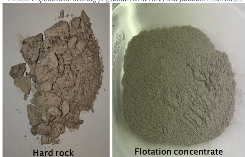
Photos 1 Spodumene bearing pegmatite (hard rock) and flotation concentrate
